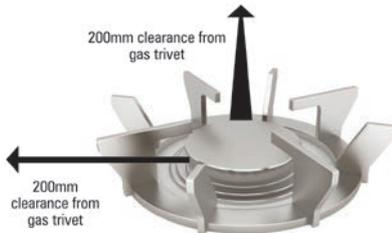
**Note: 1.** All gas appliance installations must comply with AS/NZS 5601.1: Gas Installations. **2.** All electric cooktop installations must be in accordance with the cook top manufacturer's instructions.
