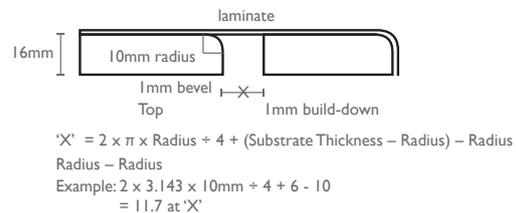
Then allow 0.5 to 1mm for additional clearance which would give a suggested dimension at "X" of 12.5mm.
