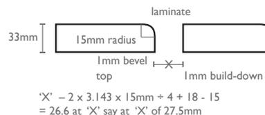
In all cases it is important that the 1mm bevel be applied to the bottom of the front edge of the benchtop section. This bevel enables additional clearance for the drop-down component to clear when being bent into position.
