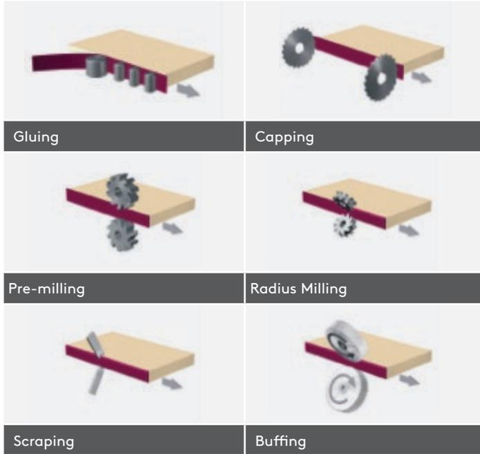
To achieve a high-quality and durable edgetape application several important processing parameters have to be considered which depend on the components used (edgetape, glue and boards), the edgbander and the ambient temperature. In order to identify the ideal conditions it is recommended that trials are carried out and that the reference values specified by the relevant manufacturer are observed.
